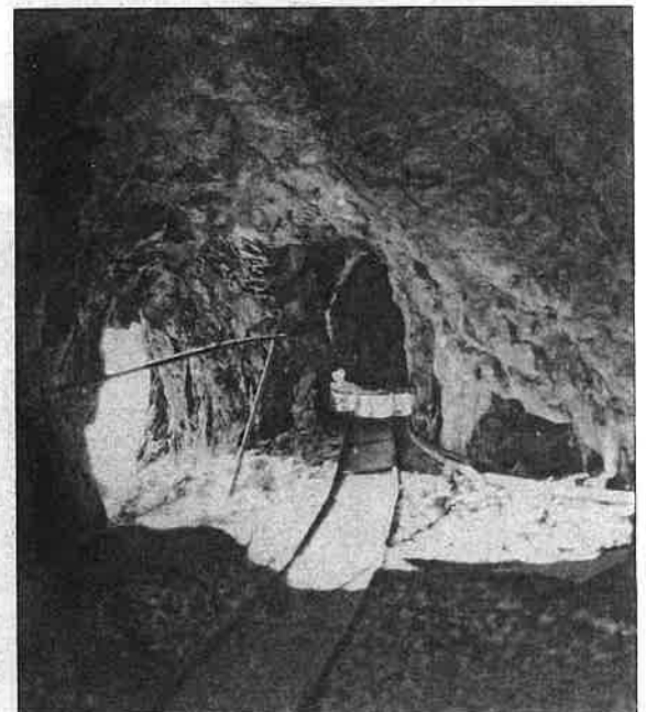
Inside one of the holes with ore cart tracks. The adit (entrance) can be seen to the left.
